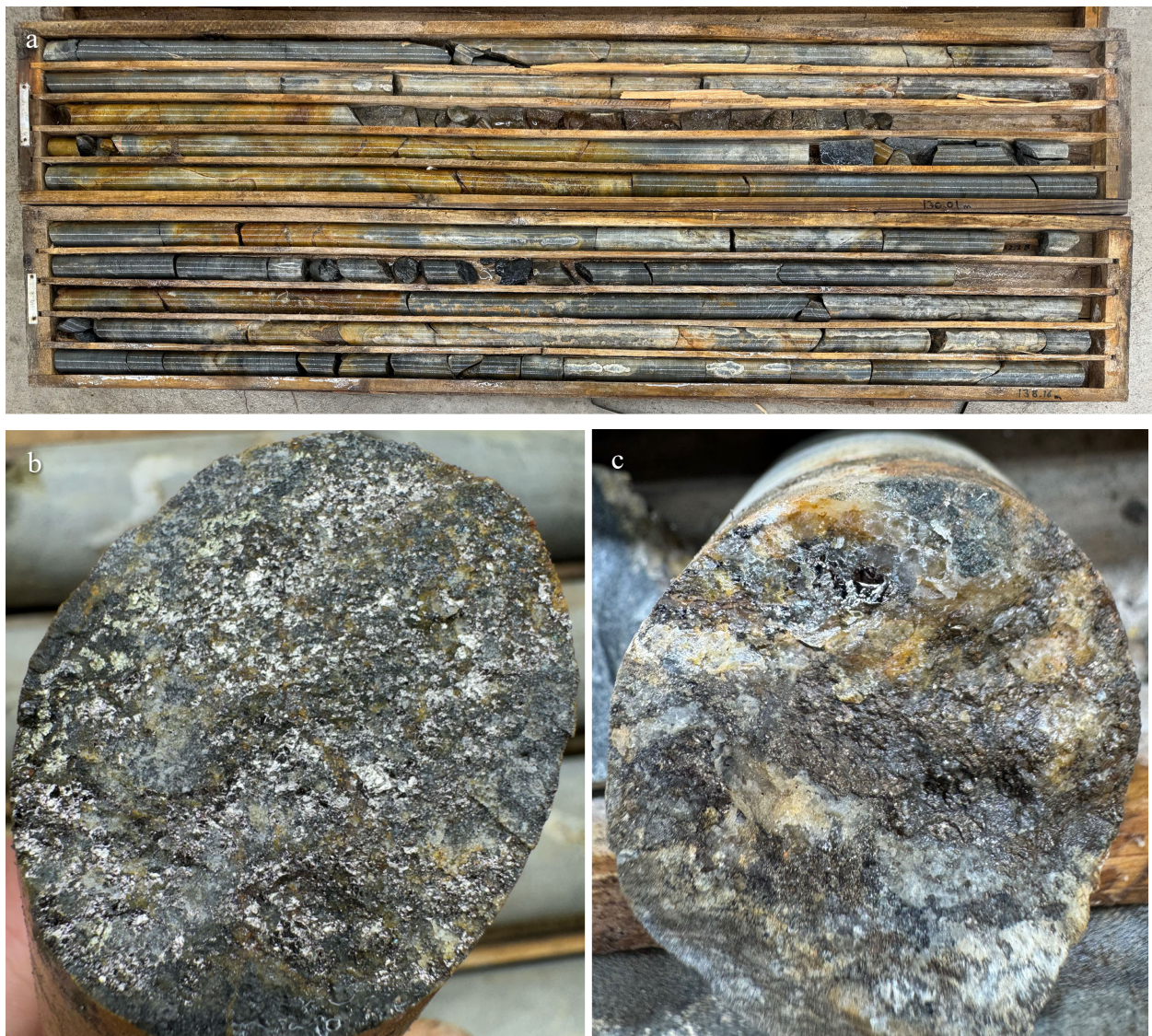
Figure 13: (a) DDH 77-30 (Central Zone) between 123.89 and 138.16m showing unsampled drill core with visible (b) chalcopyrite in a pyrrhotite-rich zone at 131m and (c) cassiterite and pyrrhotite at 117m
