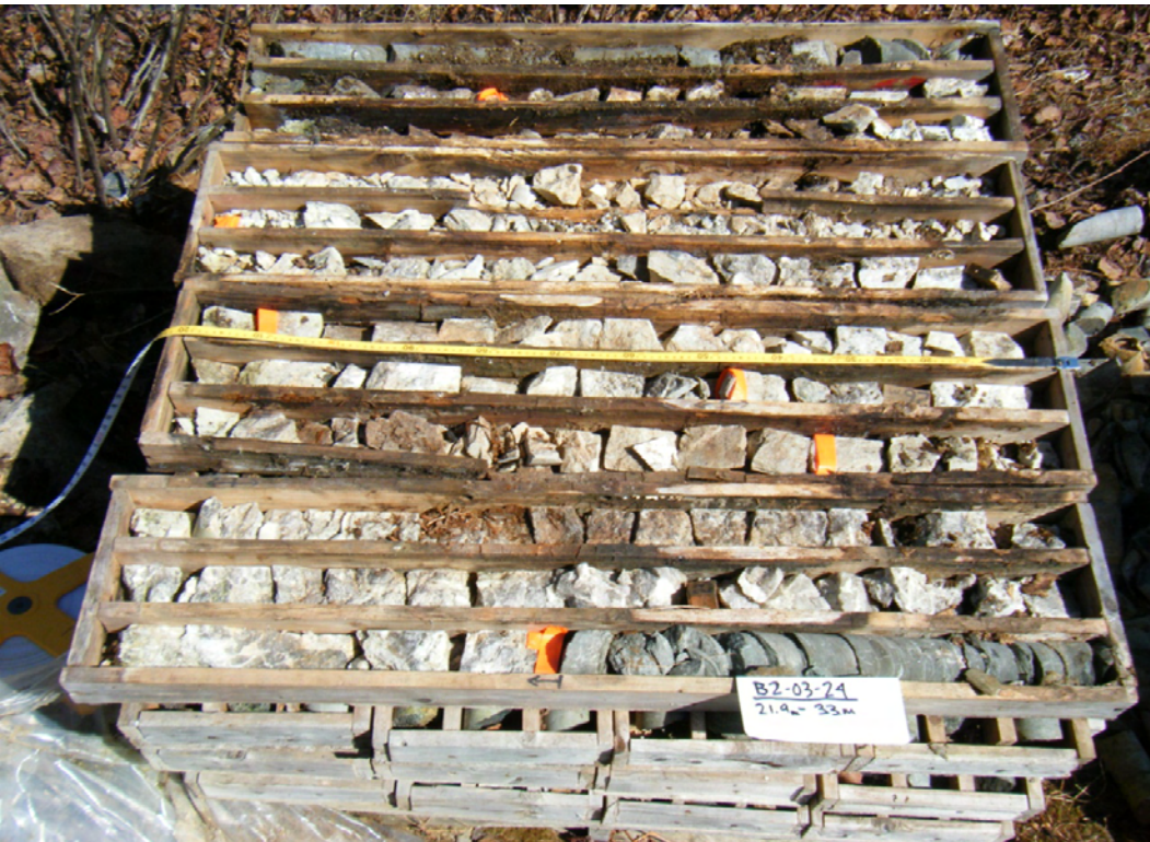
Figure 13.3: Champlain drill core showing deteriorated condition of some boxes
