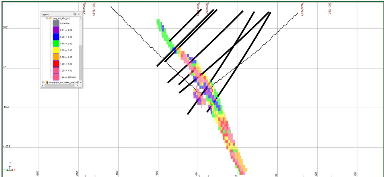
**Figure 13.17: Representative cross-section looking Northeast of the Brazil Lake Deposit South Dike ID<sup>3</sup> block grade distribution MRE pit shell (Li<sub>2</sub>O % Block Values: Purple 0.01 - 0.2 %; Blue 0.20 – 0.40 %; Green 0.40 – 0.60 %; Yellow 0.60 – 0.80 %; Orange 0.80 – 1.0 %; Red 1.0 – 1.2 %; Pink > 1.2 %. 50 m Grid Spacing)**
