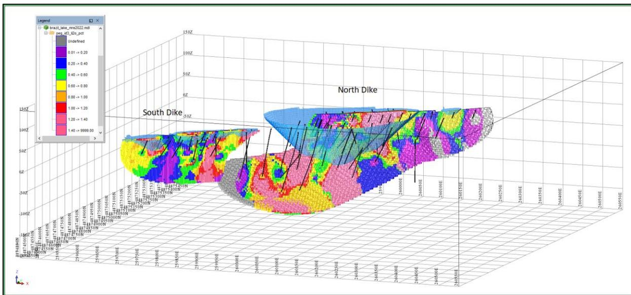
**Figure 13.16: Representative cross-section looking Northeast of the Brazil Lake Deposit North Dike ID<sup>3</sup> block grade distribution MRE pit shell (Li<sub>2</sub>O % Block Values: Purple 0.01 - 0.2 %; Blue 0.20 – 0.40 %; Green 0.40 – 0.60 %; Yellow 0.60 – 0.80 %; Orange 0.80 – 1.0 %; Red 1.0 – 1.2 %; Pink > 1.2 %. 50 m Grid Spacing)**
