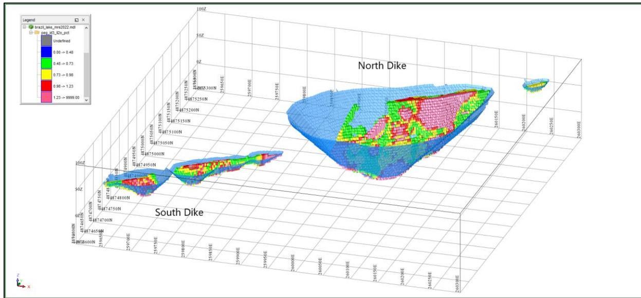
**Figure 13.19: Oblique Sectional view looking northeast of the Brazil Lake Deposit and the optimized pit shell (Li<sub>2</sub>O % Block Values: Green 0.48 – 0.73 %; Yellow 0.73 – 0.98 %; Red 0.98 – 1.23 %; Pink > 1.23 %, 25 m grid spacing)**
